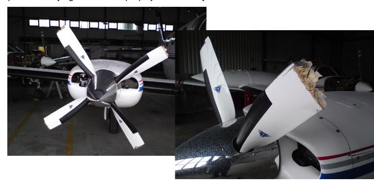
The pilot of this DA-42 was going to do a touch-n-go. At the last minute the pilot realized he forgot the landing gear. The pilot quickly added power and flew back to his home airport. The pictures are what was left of his MT Propellers at shutdown. Nearly half the blade is missing and this airplane still flew for almost 30 minutes! The pilot had no idea what had happened to the propellers until he shut down.
