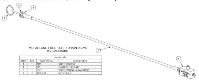
For all items not related to the installation of the McFarlane Aviation, Inc. fuel drain valve, refer to the basic airplane model service and parts manuals.
