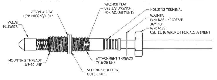
5. Thread the valve control subassembly (P/N: 6325) into the valve housing, (P/N: 6285). Continue to thread the two parts together until the outer face of the subassembly sealing shoulder is flush with, or just past, the outer face of the valve housing (see illustration below). The initial target engagement between these two parts should be between 0.000 to 0.010 inches.
