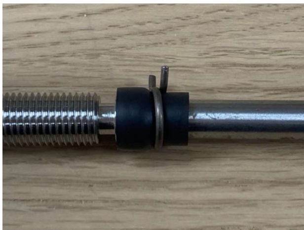
Figure 4: Correct installed position of P/N EC04 boot
