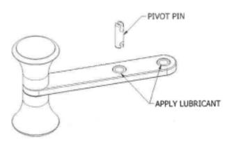
STEP 4: Apply a small amount of lubricant (moly, grease, etc) to both bushings and reinsert the pivot pin into the handle lever. Attach the new Cable Assembly (P/N 7354) to the pivot pin by sliding the wire through the groove and sliding the shank of the terminal into the pocket on the pivot pin.
