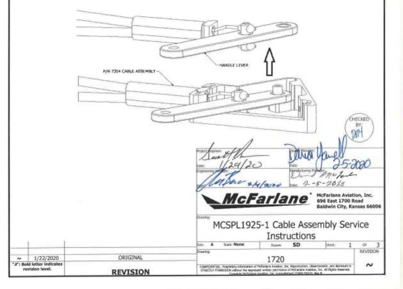
STEP 3: Disconnect the P/N 7354 Cable Assembly from the Pivot Pin and discard the old assembly. Remove the pivot pin from the housing. Clean the handle lever and pivot pin with warm soapy water and dry thoroughly.
