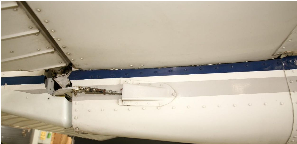
Figure 3-3, Tail Section, Tie-Down Ring Removed
