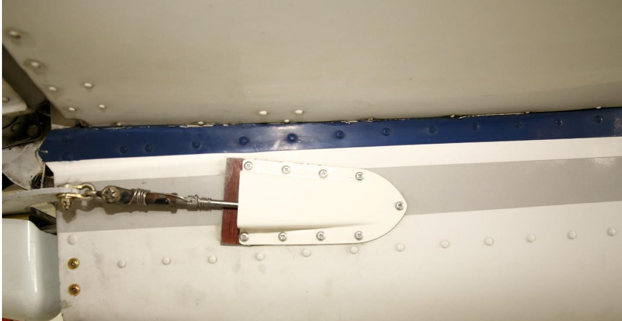
Figure 3-19, Tailcone Faring, Installed
