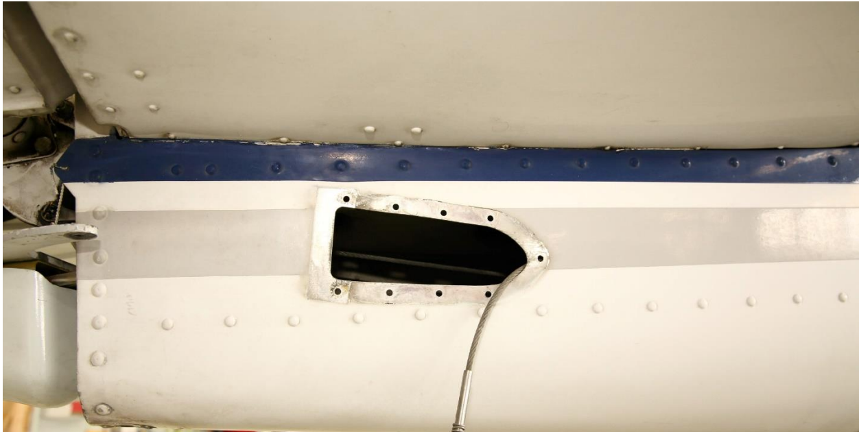
Figure 3-5, Tailcone Faring Removed and Rudder Cable Disconnected
