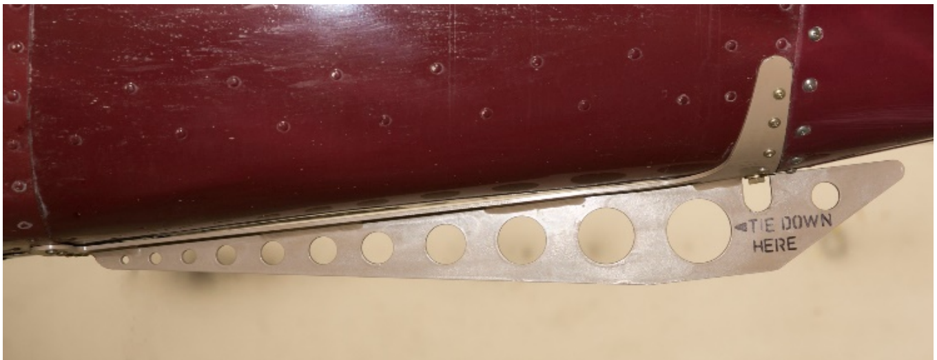
Figure 3-8, Installed Replacement Tail Tie-Down
