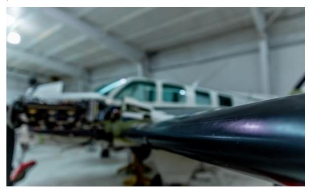
When ice begins to accumulate on the wing, the pilot will activate the boots. Air is then pumped into the flattened tubes causing them to inflate. See picture, inflated boot.
