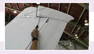
It's important to apply the material in short bursts, while turning the wands in various directions at the same time.
