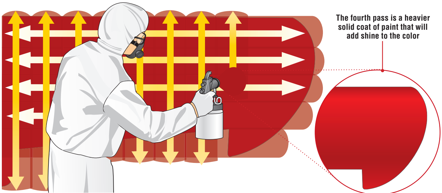
Figure 6.20 | Spraying the Fourth Pass
