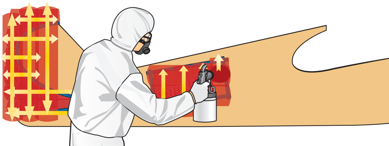
Figure 6.24 | Spray Two Complete Cross Coats
